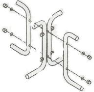
Assemble opposite legs to the "+" shaped bolt. Then attached the remaining legs.
